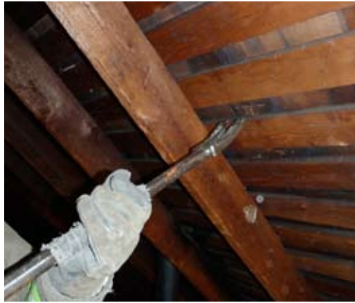
The fork can be used to open a roof on the inside during fire attack or overhaul.
